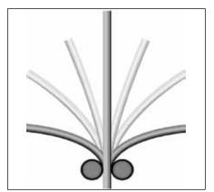
bending moment of the cable is subjected to stress and fatigue from lateral motion in these applications.
